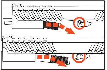
While compressed, slowly pull out the recoil spring guide at an angle, thus clearing the hop-up unit.
